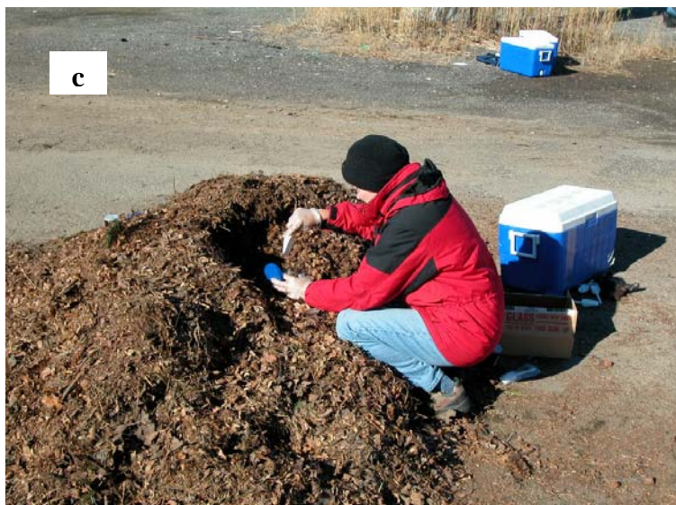
Figure 1. Photographs of sweeper waste sampling. (a) Regenerative air sweeper dumping its load.; (b) collection of samples from sifted waste stockpiles; (c) collection of samples from sweepings dumped from sweeper hoppers.
